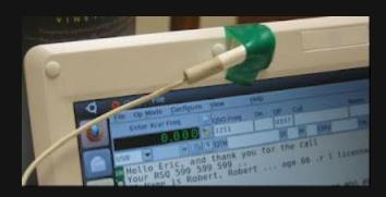
This will bring the sound of the signals from your radio to the laptop without the need for a patch cable. An electrical connection between radio and computer often causes the radio to pick-up electrical noise from the computer. By using the ear buds instead, we bring the <u>sound</u> from the radio to the computer without actually connecting the two electrically = much less computer electrical noise in the radio!
